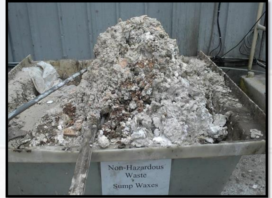
Limescale purged from boilers
