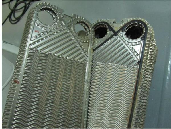
**Figure 11.** June 2013 - after installation of the HydroPath MARINE system, the plates are clean.
