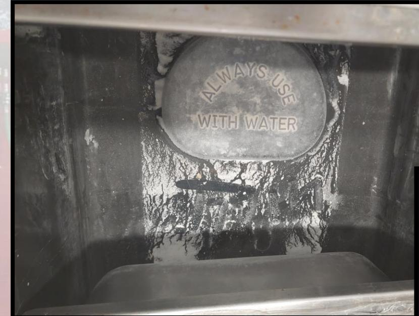
Loose scale powder collects in the bottom and rinses out easily.
